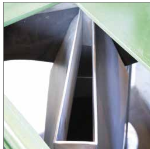
Vezin Sampler Radially Tapered Cutter
