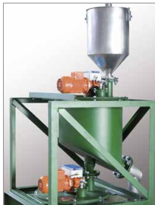
Vezin Sampler with Stainless Steel Surge Hopper
